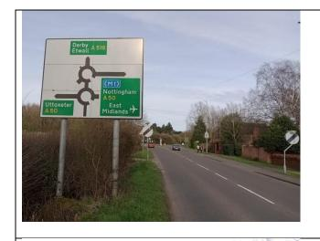
When approaching from the Hilton direction motorists could be confused by the direction sign as the righthand 'stub' aligns with the wording for the A50 to Nottingham.
